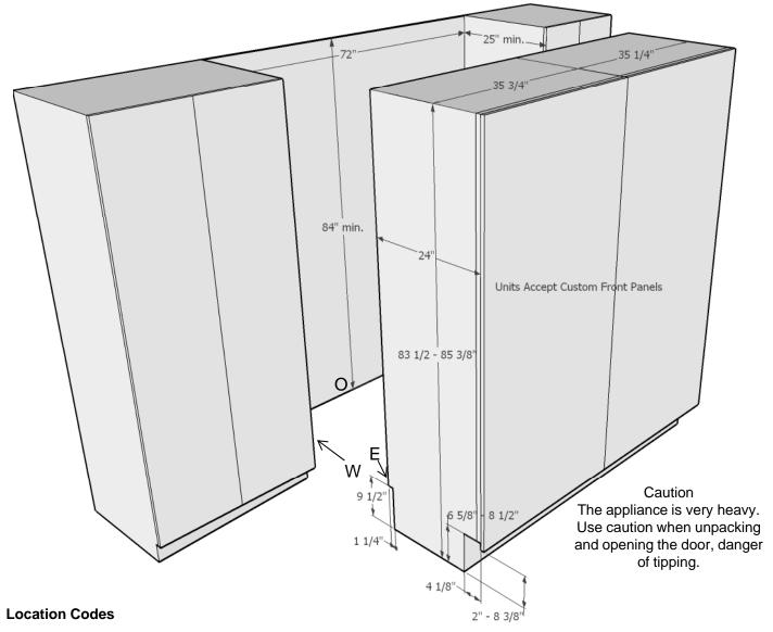
E- 5 foot – 120 Volt – 15 A 3-wire molded plug power supply connects lower left rear.
